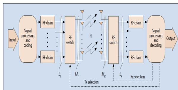
Figure 1: Antenna selection in MIMO system
