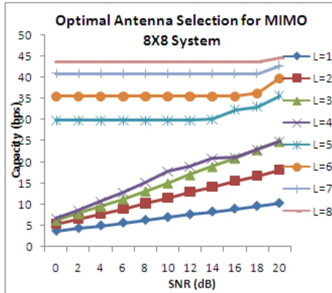
Figure 2: capacity of optimal Antenna selection for 8X8 MIMO system
